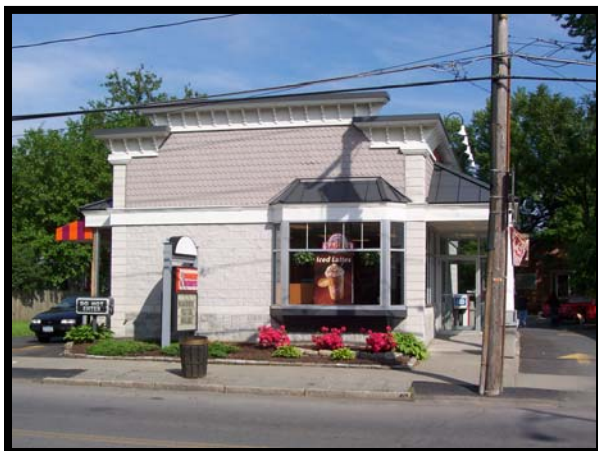
Above: Better Main Street building type: very small setback, parking is to the side and in back, moderate fenestration ratio, more traditional looking building materials (Note: example pictured is a corporate chain restaurant) (Broadway, Rensselaer, NY)
