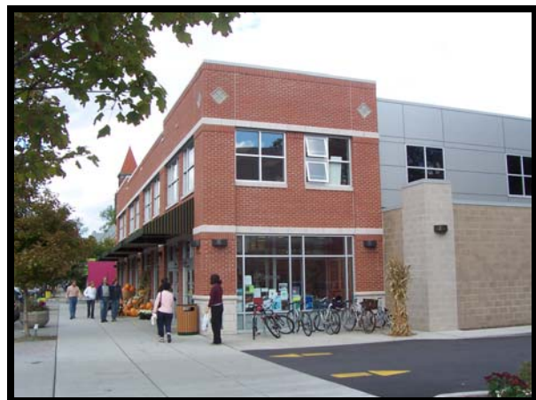
Above: Even better Main Street building type: no setback, parking is to the side and in back, building is two stories tall, high fenestration ratio, traditional looking building materials (Elmwood Avenue, Buffalo, NY)
