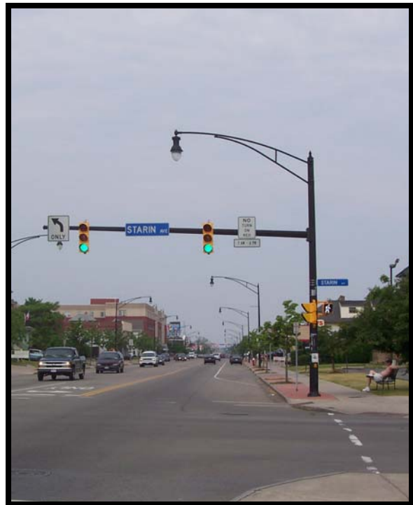
Above: Contemporary light poles, painted black, and utilizing more decorative hanging light fixtures. The height of the poles and repetitive spacing pattern help define the streetscape in the absence of taller buildings close to the sidewalk. Hertel Avenue, Buffalo, NY
