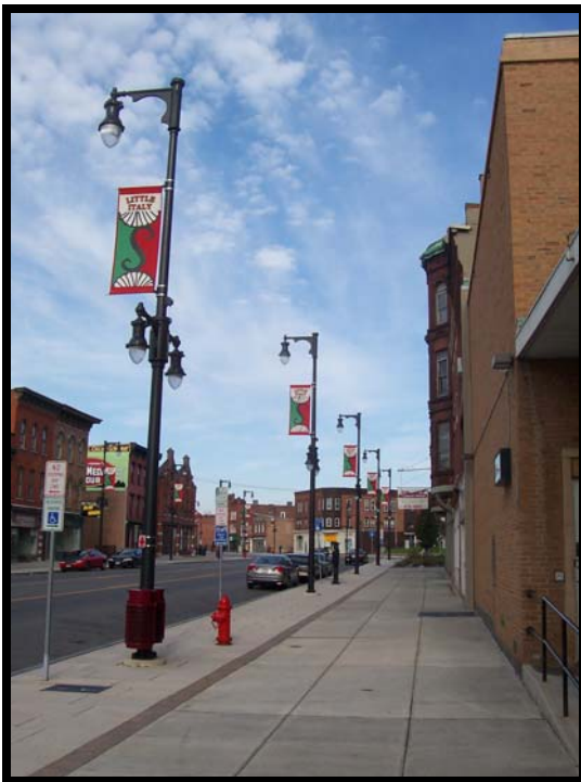
Above: Light poles that accommodate both taller, more “auto-oriented” light fixtures and lower pedestrian scaled light fixtures. North Salina Street, Syracuse, NY
